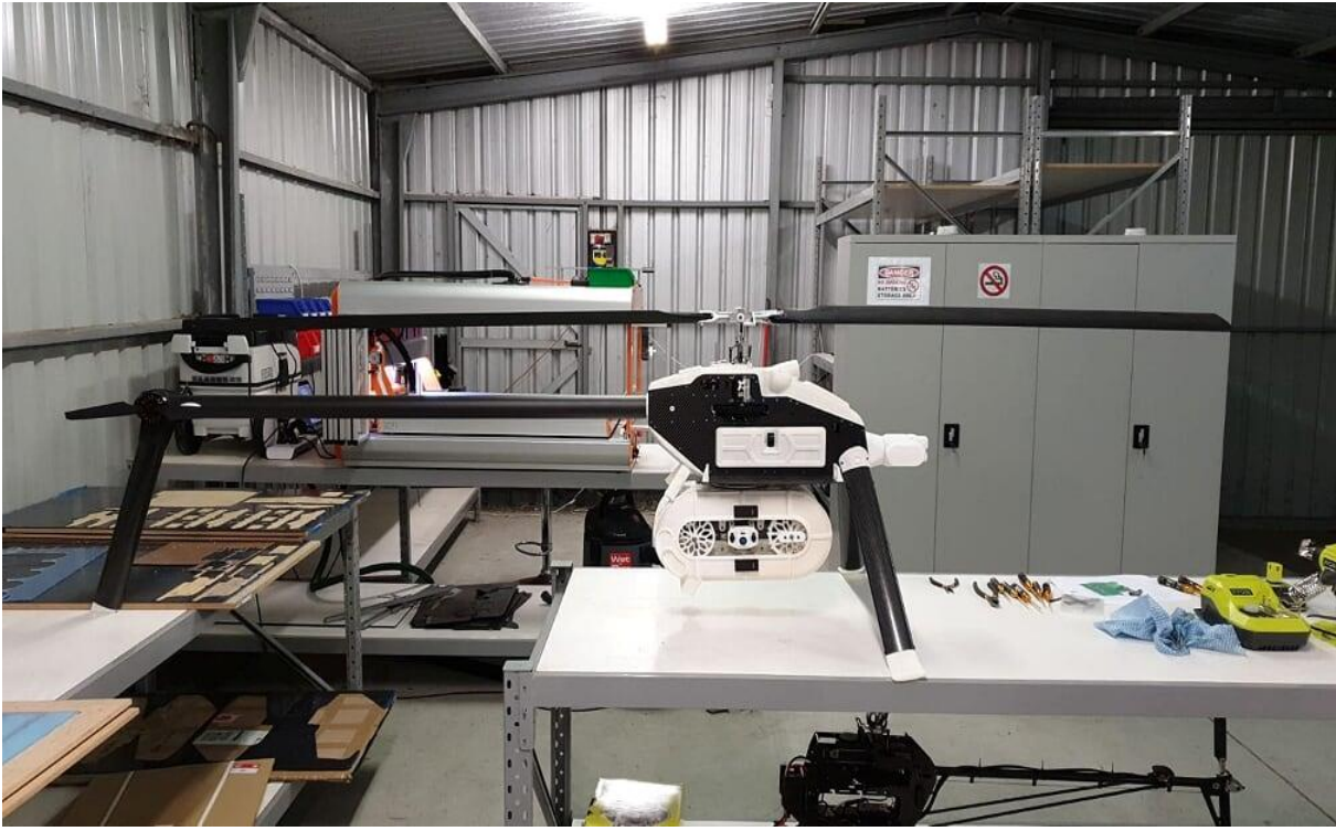
Autonomous Technology Drone Fitted with Bait Delivery System
